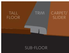
**END CAP** (often times called Square Edge or Threshold) is most commonly used when butting up to carpet or a sliding glass door.
