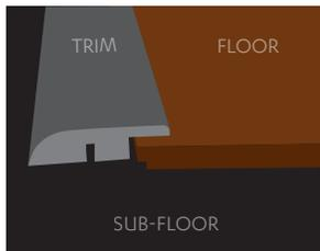
**REDUCER** is used when ending the flooring onto a surface such as concrete.
