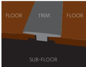
**T-MOLD** is used when joining two floors of equal height, such as in a doorway, between two rooms or in a large area where the maximum length/width is exceeded.
