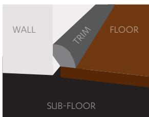
**QUARTER ROUND** is most commonly applied to cover the expansion gap between the flooring and the wall.
