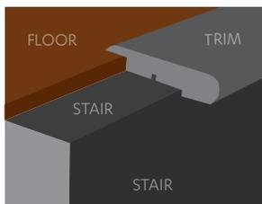
**STAIR NOSE** is used when ending flooring at the top of either a landing or downward staircase.
